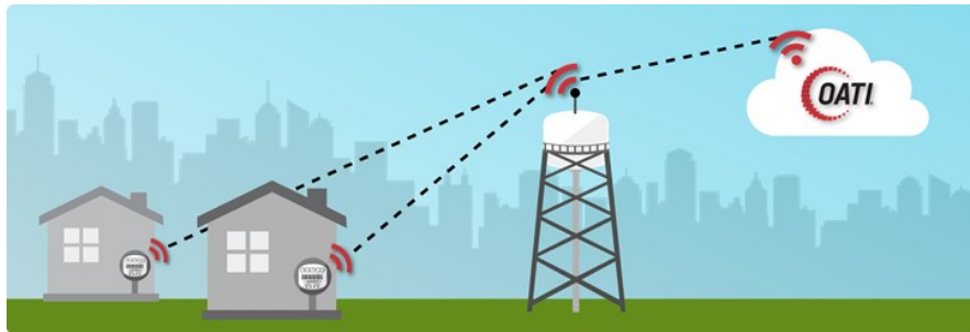
Figure 1 – Image depicting the OATI network reading AMI meters.
